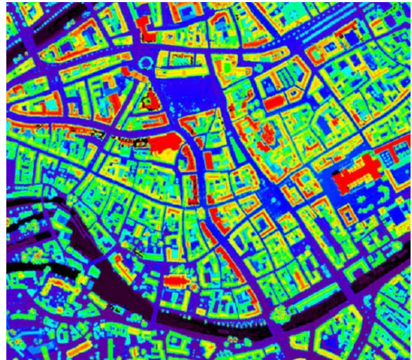
France, Strasbourg: colour-coded elevation model of the city center
