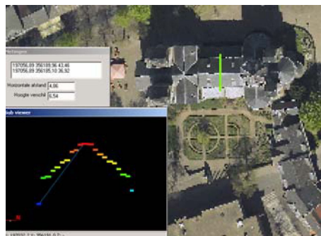
3D-Viewer: profile view of building in DSM
